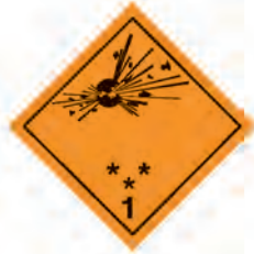
(No. 1) Divisions 1.1, 1.2 and 1.3 Symbol (exploding bomb): black; Background: orange; Figure "1" in bottom corner
