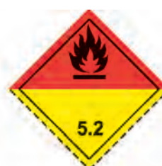
(Nr. 5.2) Symbol (flame): black or white; Background: upper half red; lower half yellow; Figure "5.2" in bottom corner
