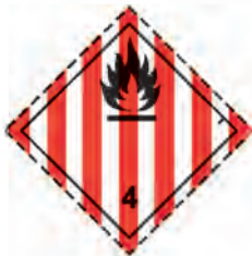
(No. 4.1) Symbol (flame): black; Background: white with seven vertical red stripes; Figure "4" in bot- tom corner
