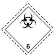
(No. 6.2) The lower half of the label may bear the inscriptions: 'INFECTIOUS SUBSTANCE' and 'In the case of damage or leakage immediately notify Public Health Authority'; Symbol (three crescents superimposed on a circle) and inscriptions: black; Background: white; Figure '6' in bottom corner
